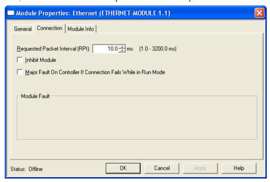
After clicking OK, the new PLCIO tag will be available in the list of Controller Tags on the PLC. You can view the input and output data on the PLC side by monitoring tags PLCIO:I and PLCIO:O, respectively. Data will be available only when the connection from the PLC to your PLCIO program is fully established.
