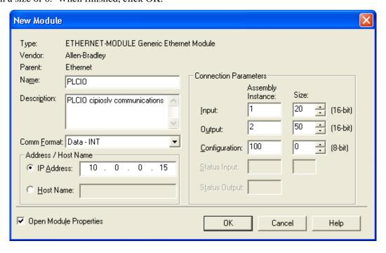
Next, select a reasonable RPI (Requested Packet Interval) for this communications channel and click OK. The RPI denotes how often the PLC will send output data to PLCIO, and how often it expects to receive input data from PLCIO. The PLCIO application must attempt to do a plc\_write() once every RPI in order to keep the connection established. If the PLC does not receive a message within 4 times the specified RPI, then the PLC will close and reopen the connection to *enipd*.
