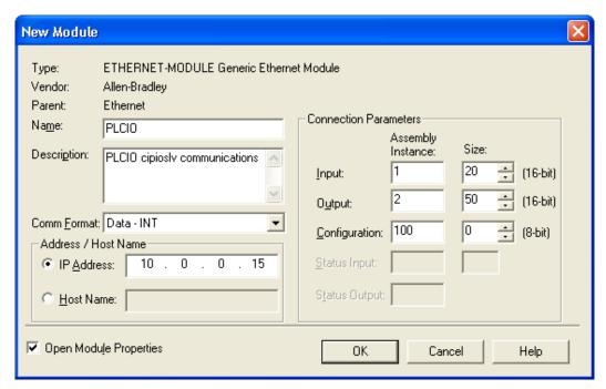
Next, select a reasonable RPI (Requested Packet Interval) for this communications channel and click OK. The RPI denotes how often the PLC will send output data to PLCIO, and how often it expects to receive input data from PLCIO. The PLCIO application must attempt to do a plc\_write() once every RPI in order to keep the connection established. If the PLC does not receive a message within 4 times the specified RPI, then the PLC will close and reopen the connection to enipd.
