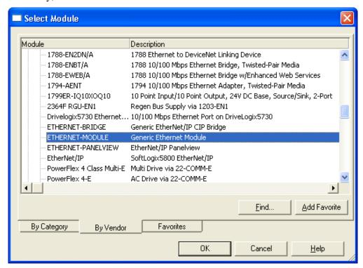
Next, fill in the Name and Description the same as you would for a standard I/O Bus Terminal. Select any non-status communications format (INT, DINT, REAL, etc.) that matches the data type you intend to transmit. Type in the IP Address of the target computer that is running PLCIO.
